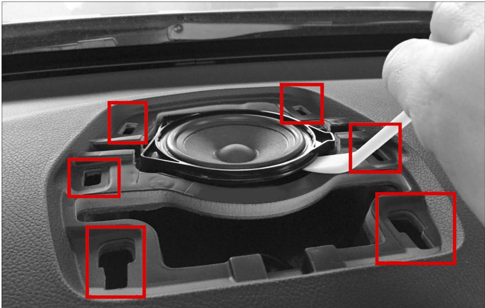
The original speaker is plugged in at three points on the panel. If necessary, use a plastic wedge to lever out the speaker. To unlock the connectors, use either a small screwdriver or a paper clip. Connect the supplied crossover to the original connection cable (gray / gray black) and the other end to one of the two connection terminals of the EM-MBC1.
